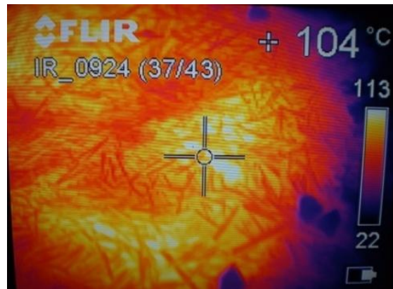
Figure 4: Thermogram of grinding elements after exiting the chamber.
